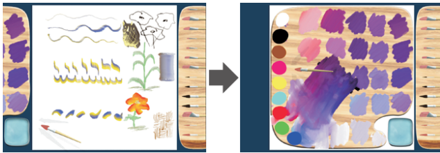
Figure 4: Graphical User Interface: The virtual canvas with the brush rack and a portion of the palette (LEFT); the brush rack and the palette for color mixing (RIGHT).
